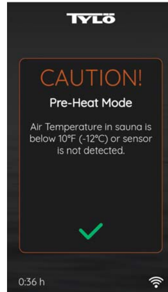
Figure 29. CAUTION Pre-Heat Mode Screen
