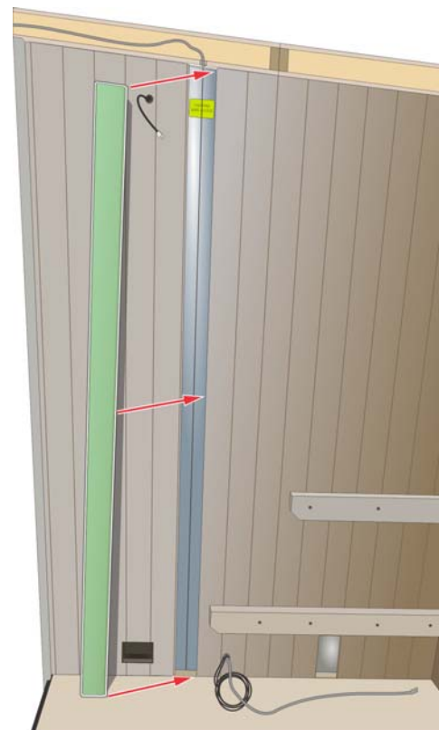
Figure 21. Taping Vapor Barrier and Installing Plank
